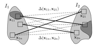
Fig. 1. Illustration of the graph considered when computing the dissimilarity between two images,  $I_1$  and  $I_2$ , in (4). All edges have an associated weight  $\Delta(\mathbf{x}_{1i}, \mathbf{x}_{2j})$  that expresses the textural dissimilarity between the two corresponding ROIs  $\mathbf{x}_{1i}$  and  $\mathbf{x}_{2j}$ . The edges in the perfect matching with minimum weight  $M^*$  are shown as solid lines, and the remaining edges, not in  $M^*$ , are shown as dashed lines.
